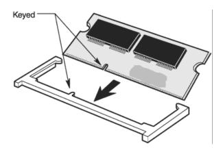
Figure 39. SODIMM Installation – Keyed Slots
